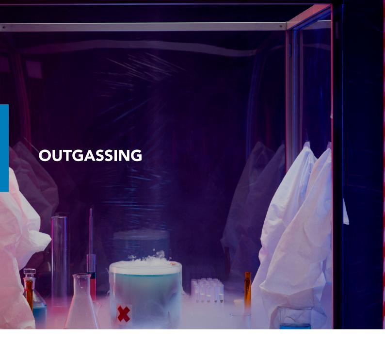
Outgassing is the slow release of trapped moisture/oxygen from materials brought into the glove box. Over time, this can change the internal atmosphere.
