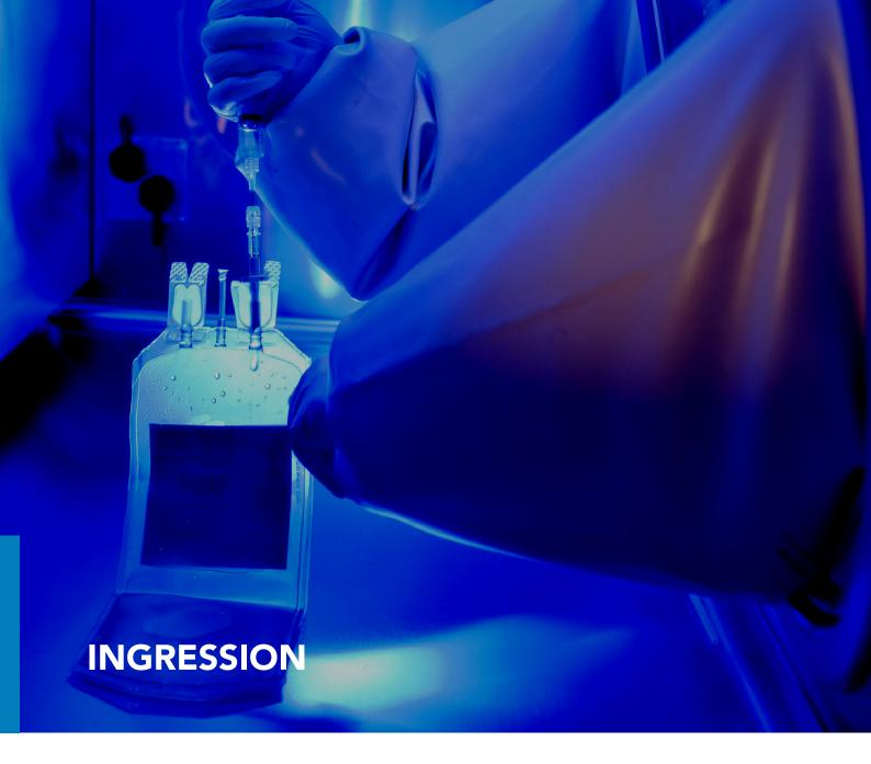
Ingress, in the case of glove boxes, is the diffusion of unwanted oxygen and water into a sealed chamber.
