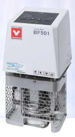
Immersion temperature devices and coolers differ from water and oil baths in one huge way: instead of immersing the sample within a water or oil bath, immersion devices and coolers are placed in a basin which is filled with water or oil, and the sample is placed in the basin when the required temperature is reached. Their applications are quite different too. Sometimes, immersion devices and coolers are used to readjust the temperature of a small quantity of a previously heated or cooled sample.
