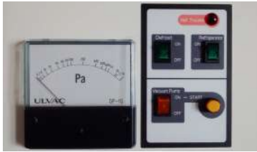
Pirani Vacuum Gauge and Control Panel
