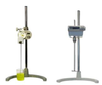
...large volumes or high-viscosity substances. They often feature useful safety features, like sensors that shut down the motor if it overheats (which can happen with highly viscous liquids).
