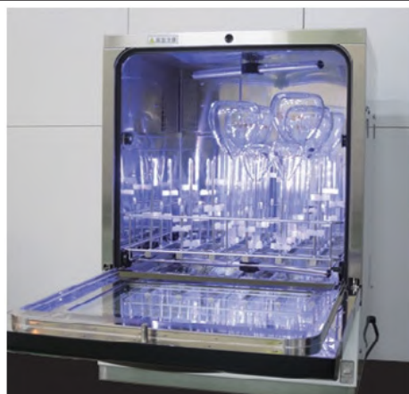
Jet rack, Slide-type A5 (291063) Flask not included The end of each pipe is a nozzle
