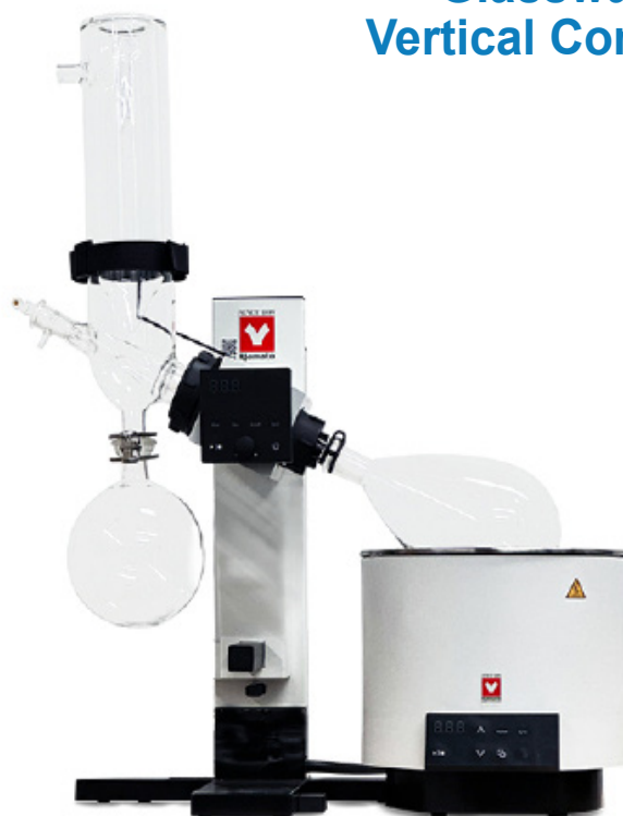
Glassware C Cold-finger, Vertical Condenser
